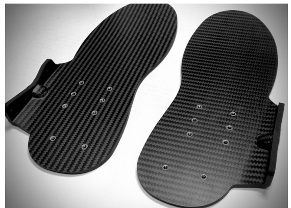
Finished carbon fiber parts produced from the 3D printed layup and trim tools.
